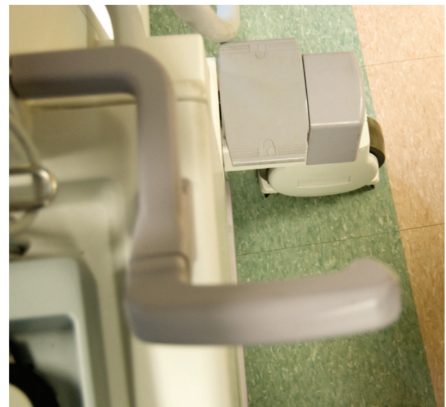
Fig. 14. The handles on a C-arm help steer the base of the unit. Note how the handle and wheel are turned in the same direction. Also note the pedal brake associated with the wheel.
