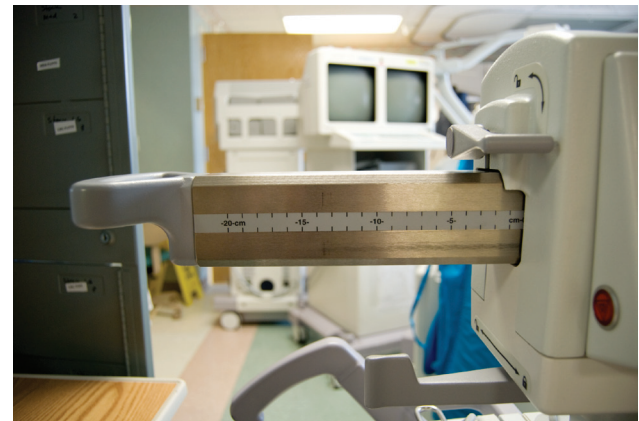
Fig. 13. The C-arm can move forward and backward in relation to the base of the unit, a feature called telescoping.
