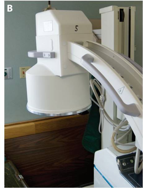
Fig 5. A. Diagram of an image intensifier used in a mobile fluoroscopy system. B. The image intensifier of a mobile fluoroscopy unit. The image intensifier increases the brightness of the fluoroscopic image.
