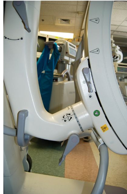
Fig 10. Example of the brake handles and lock indicators on a mobile fluoroscopy unit.
