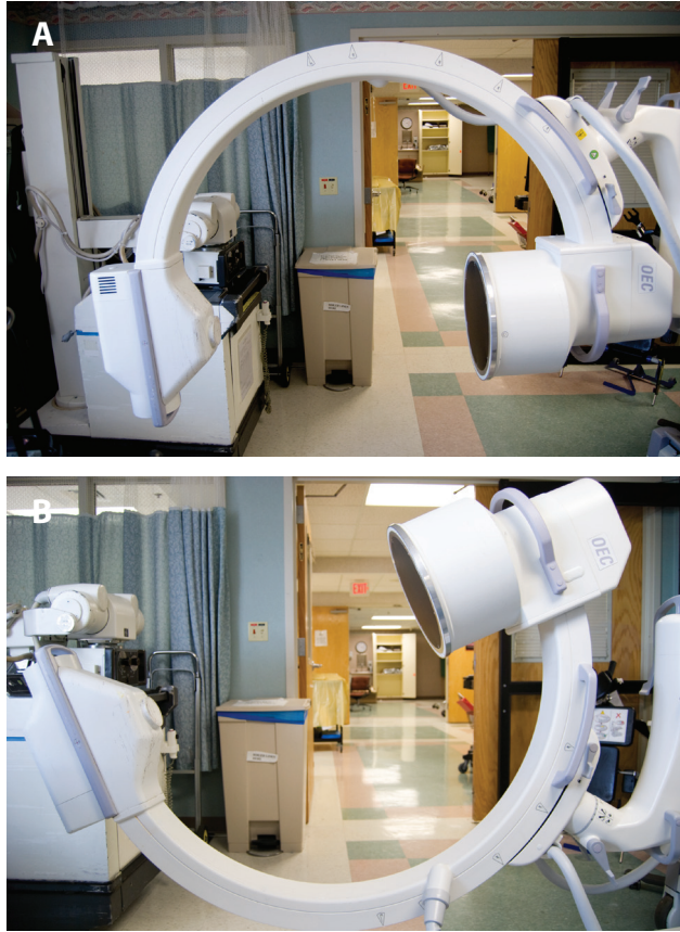
Fig. 11. During orbital rotation, the x-ray tube and image intensifier or flat panel detector glide along the natural curve of the C arm. A. Overscan. B. Underscan.
