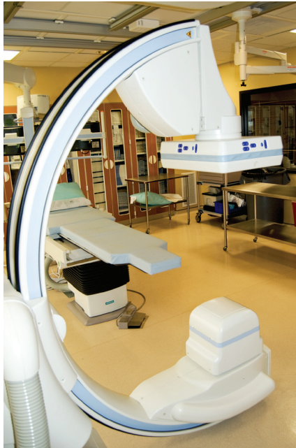
Fig. 6. Flat panel detector. The flat panel detector may one day replace the image intensifier as the standard image receptor in the mobile fluoroscopic system.
