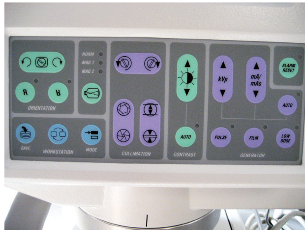
Fig. 2. Above. Mobile fluoroscopy control panel. This control panel is separated into 5 different categories: orientation, collimation, contrast, generator and workstation.
