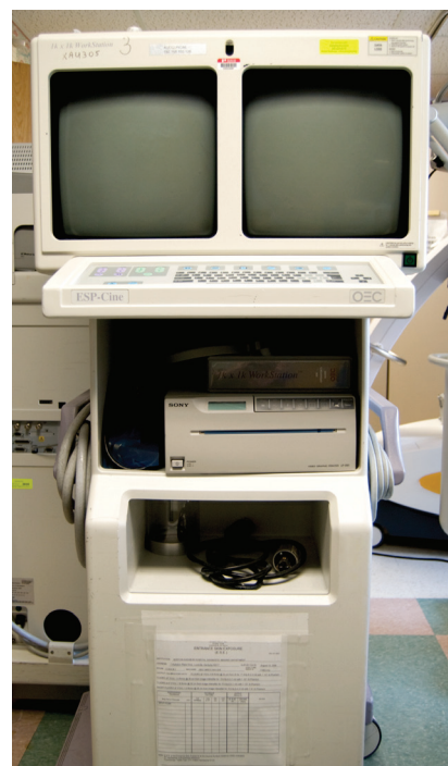
Fig. 2. Above. Mobile fluoroscopy control panel. This control panel is separated into 5 different categories: orientation, collimation, contrast, generator and workstation.
